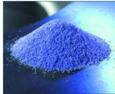
Microcrystalline sintered alumina Identification: EB or EX
