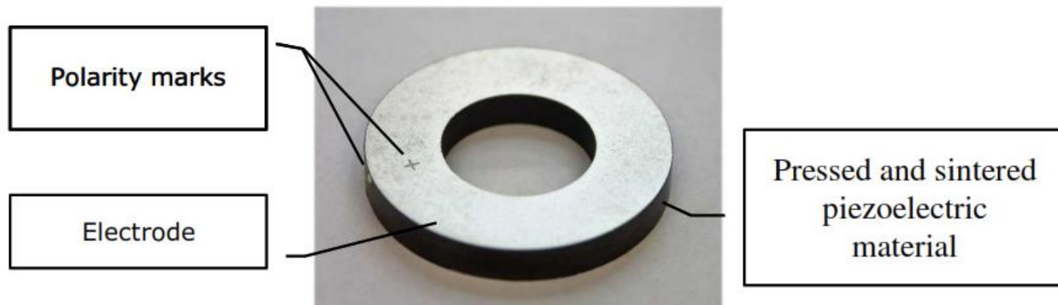
Figure 1- Typical piezoelectric ceramic for ultrasonic welding converters.
