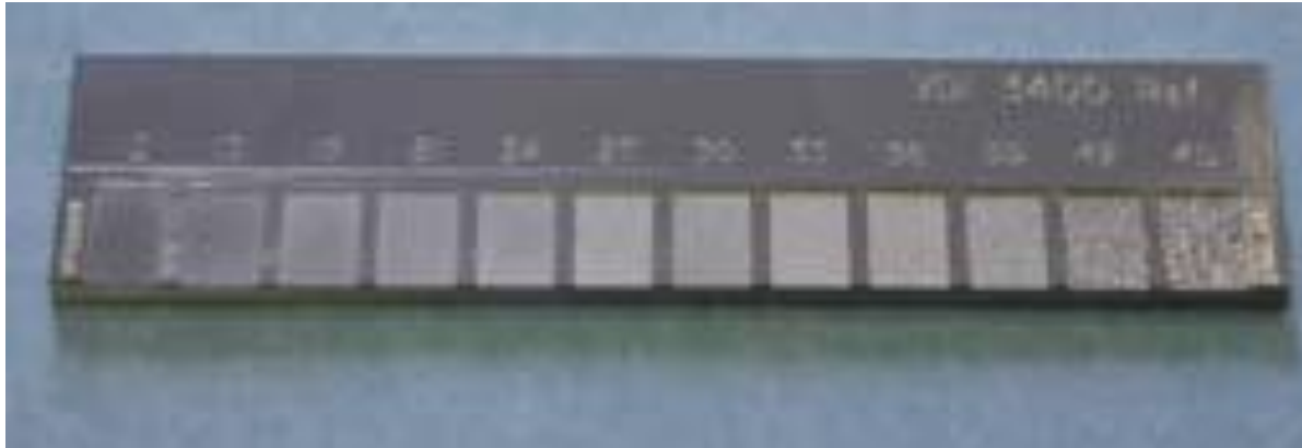
Surface finish comparison chart in EDM Standard: VDI 3400
