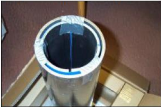
Step 3: fill gap with epoxy
