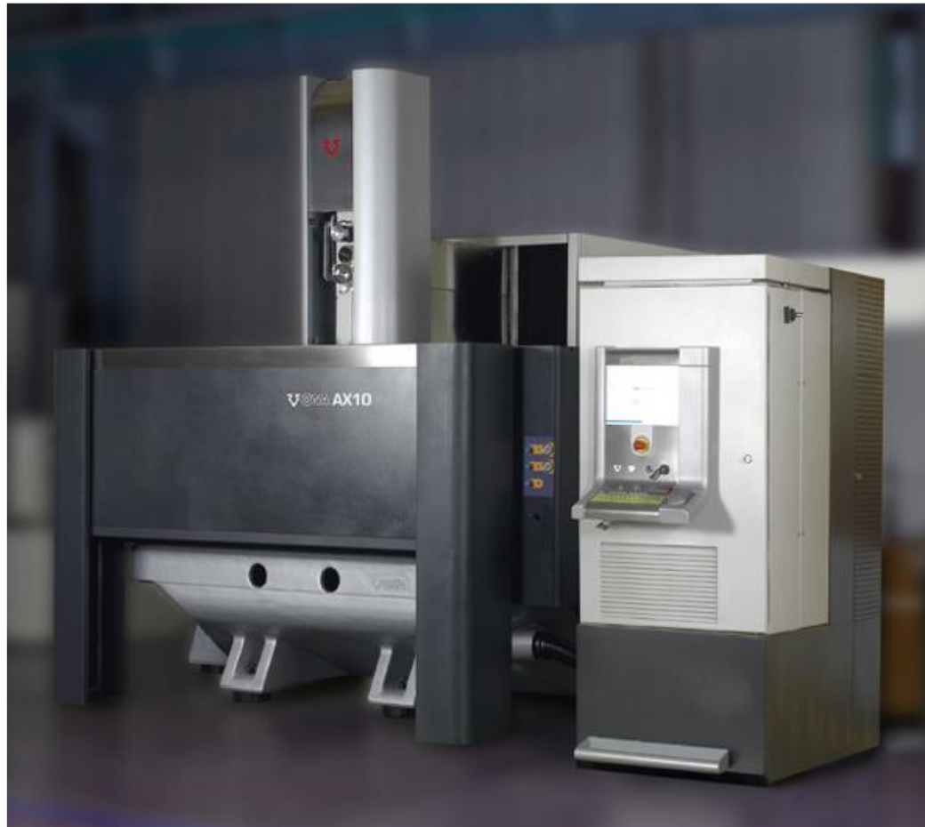
ONA AX-10 for the cutting of large thickness parts
